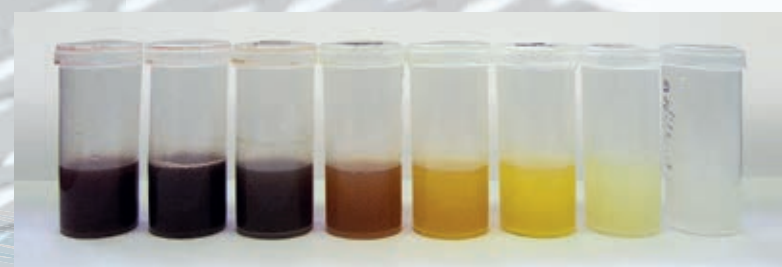
Wastewater treated with diamond anodes
