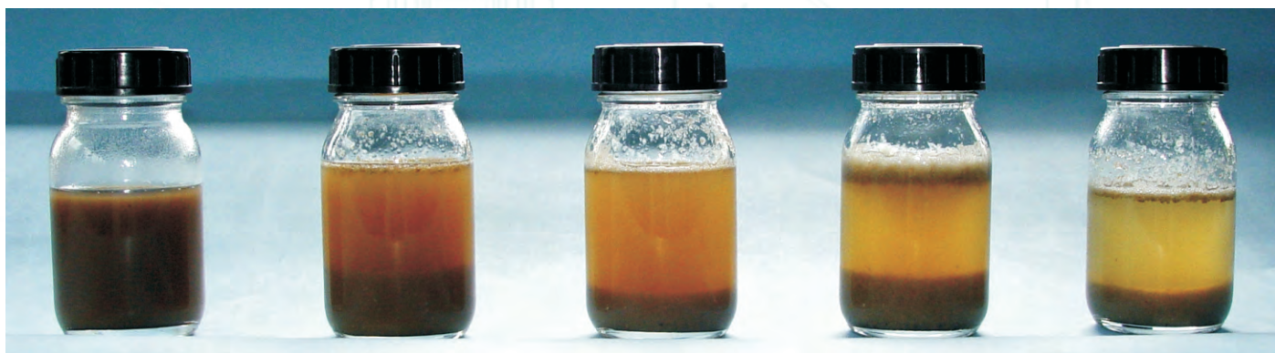
CLEANING OF HEAVILY POLLUTED WASTE WATER BY DIAMOND ELECTRODES AFTER DIFFERENT TREATMENT TIMES.
